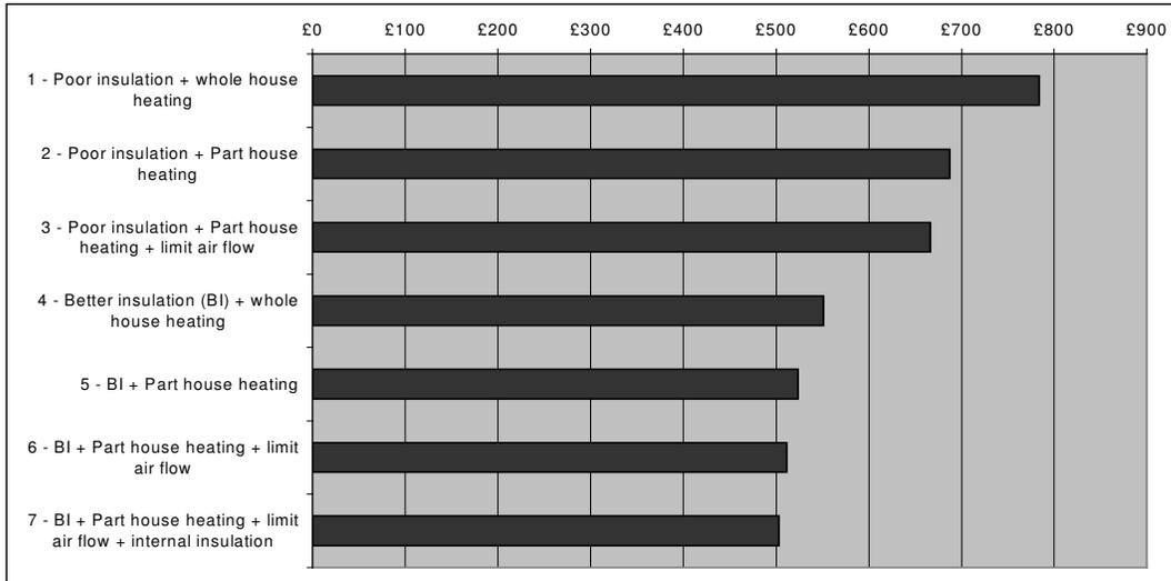
**Figure 6: Annual total energy costs for 6 example houses with different levels of heating, insulation and internal airflow assuming a single occupant**
